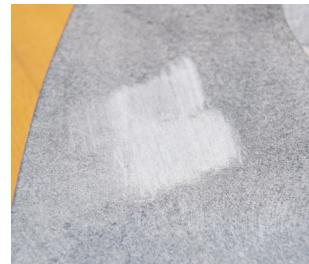
Regularly remove the loose dust with a dry cloth. When the scratch/stain is only slightly visible, you are ready to use the grit P220 for surface finishing.
